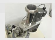
Automatic hopper feeder prevents test substance from sticking inside and provides continuous and steady feed supply to generation turntable.
